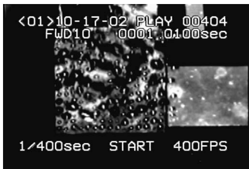
Fig. 3. Still image showing 100% nucleation at ONB for surface 1.
